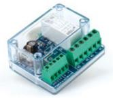
**FULL RELAY** - 12/24 Vdc/Vac relay interface board, 40 mA @ 24 Vdc power supply max consumption. Opto-isolated input 3 - 30 Vdc/Vac max 10 mA. 1 DPDT (Double Pole, Double Throw) output with dry contact with maximum 8 A 250 Vdc/Vac. 2 8 Ah outputs or 1 16 Ah output. Dimensions: (HxLxD) 60x48x26 mm - weight: 48 gr.
